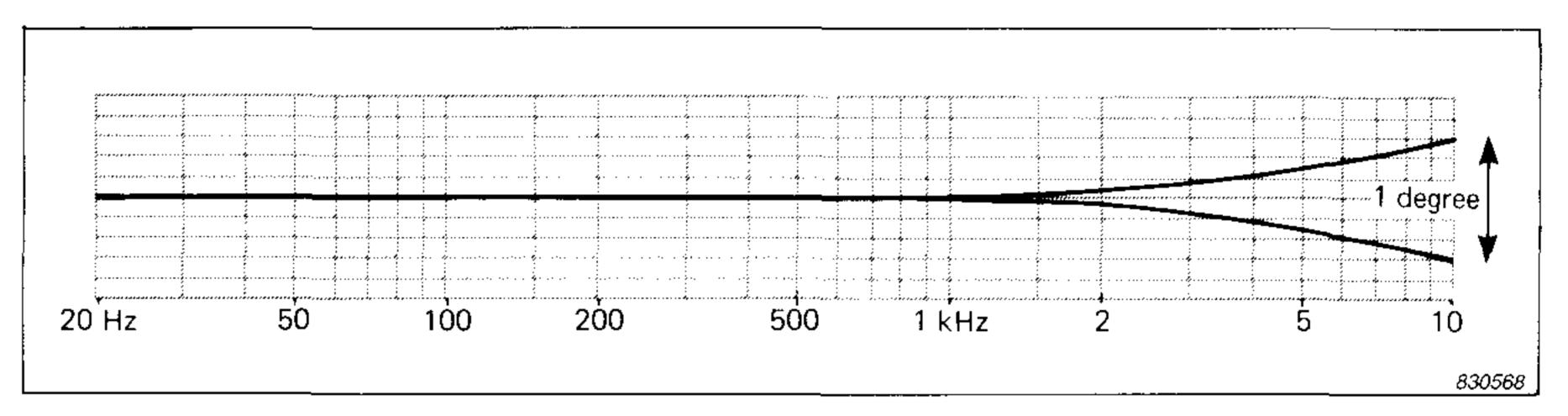
Fig.4. Typical relative phase-mismatch between two channels using FM recording with optimal azimuth adjustment
