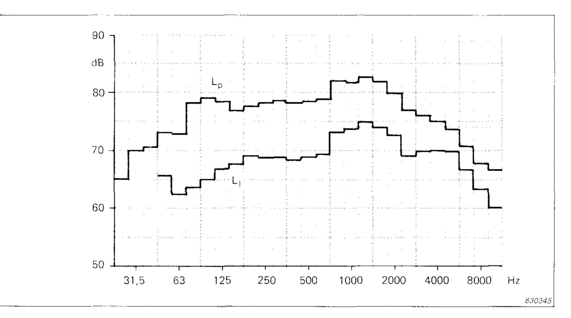
The linear averaging time was 32 seconds in each measuring point, and channels 2 and 3 equipped with FM-units ZM 0053 were used. The FM-units were switched to AC-mode to avoid low frequency overload of the input amplifiers. A pistonphone reference signal was recorded in Fig.15. L<sub>p</sub> and L<sub>l</sub> averaged over 10 measurement positions. The reactivity of the sound field is the difference between the two spectra
