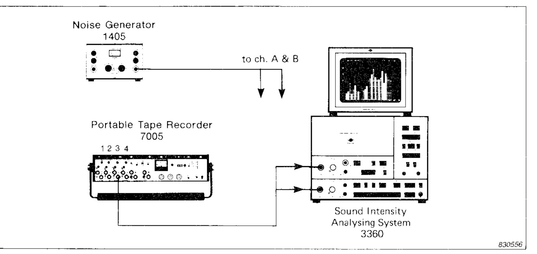
Fig.9. The dynamic range of the analyser alone (without the probe) can be checked by putting the
