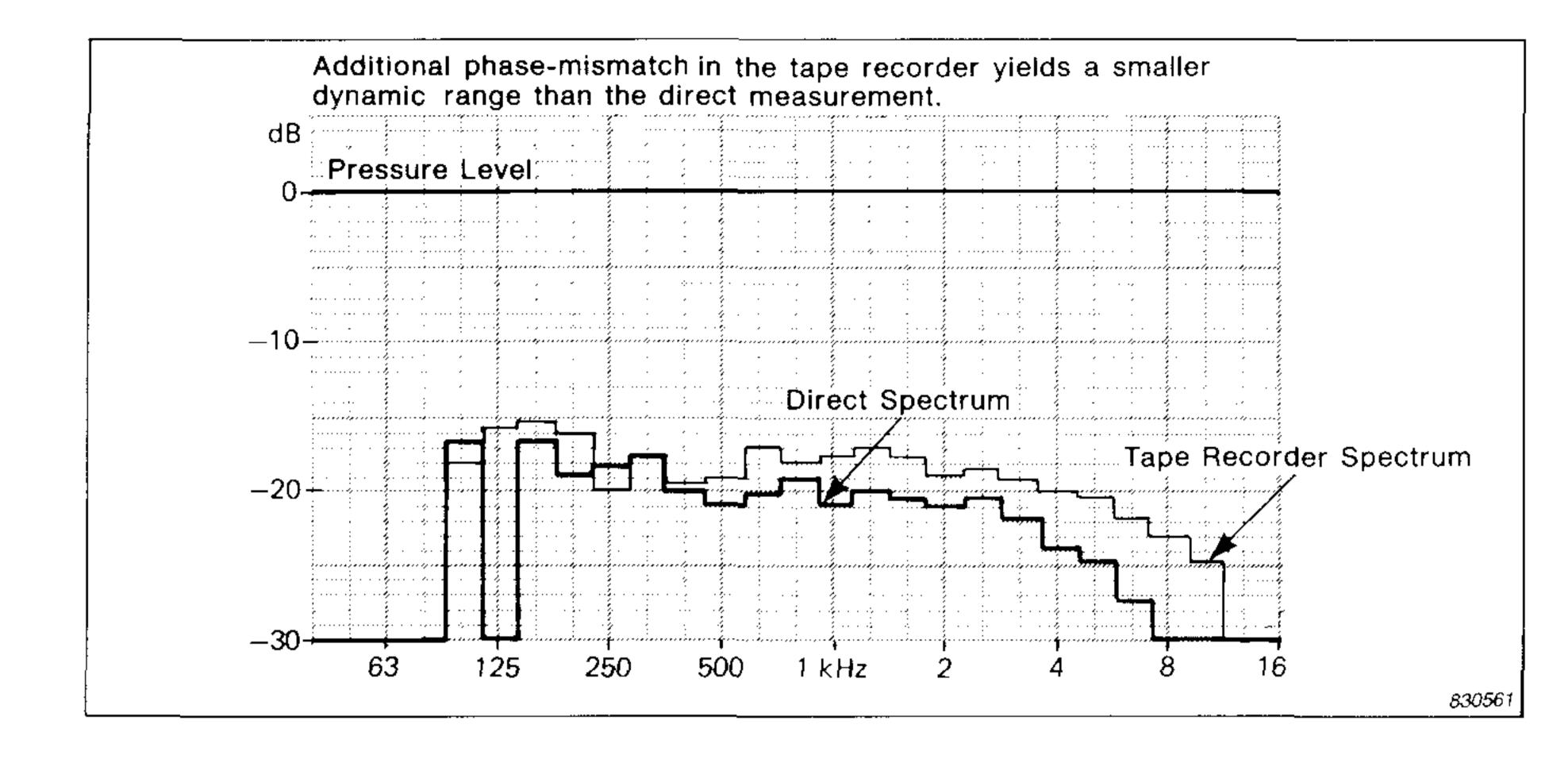
This technique enables all 4 channels to be used and then to be phase-matched in pairs before reproduction. The phase matching is optimal, and the measurements can be performed without previous adjustments, although reference signals have of course to be recorded.
