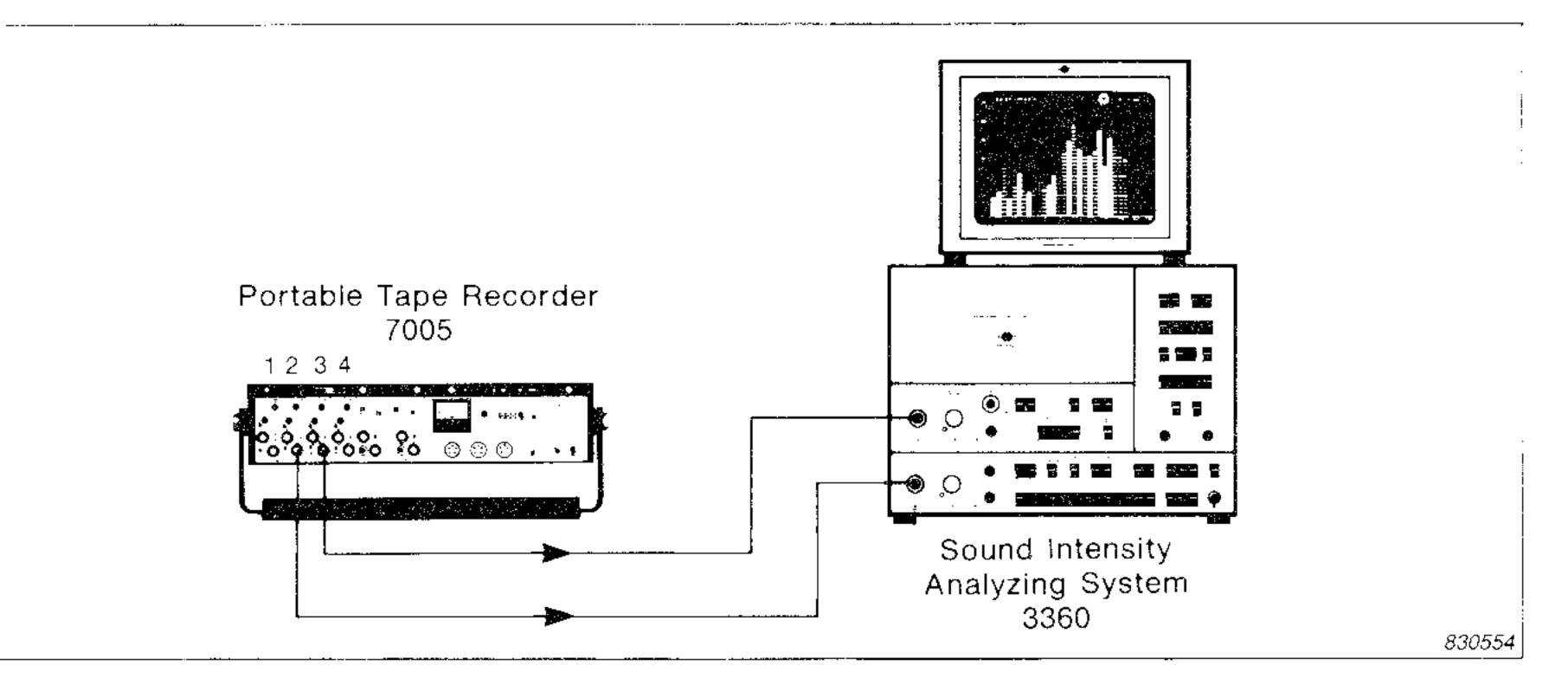
Fig.10. Set-up for analysis of the tape recorded Intensity measurement
