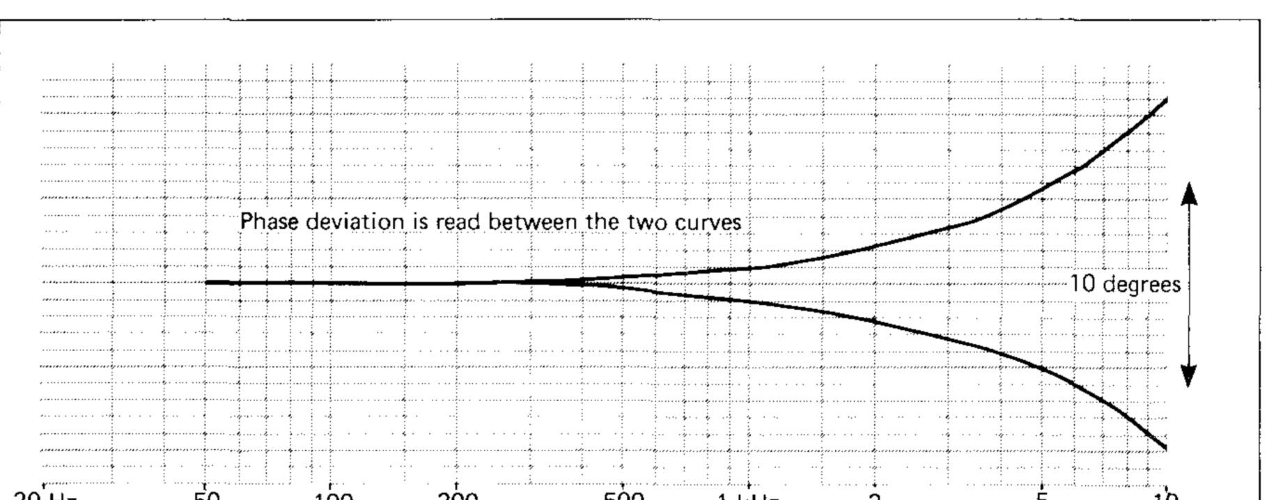
two channels using direct recording is illustrated in Fig.3 where it is seen that the low frequency phase response is worse than for the inputoutput amplifiers alone (Fig.2a). Fig.3 also shows the poor phase response at the midrange frequencies due to direct recording. To summarise, it is difficult to obtain a good
